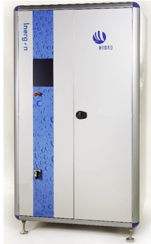
FIGURE 2.15 PEM electrolyzer by Yara (Norsk Hydro Electrolysers). Productivity, 10\text{ Nm}^3\text{ H}_2/\text{h} ; electric power consumption, 4.4\text{ kWh/m}^3 ; output pressure, 3.0\text{ MPa} ; hydrogen purity, 99.9\% ( \text{O}_2 as main impurity). (For color version of this figure, the reader is referred to the online version of this book.)
