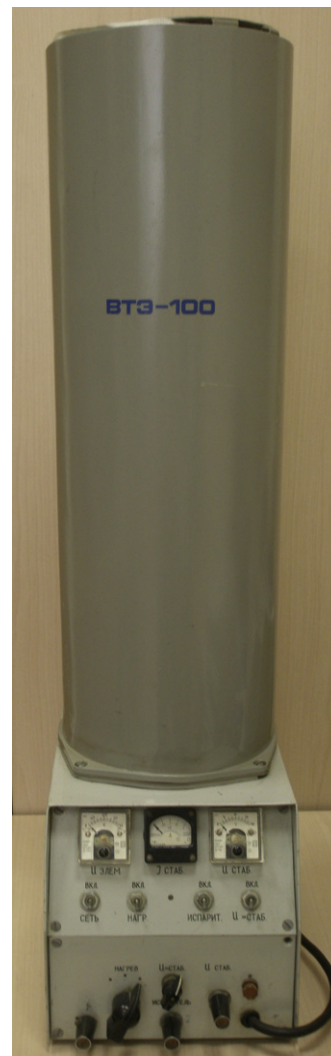
FIGURE 2.24 High-temperature electrolysis for 100 L of hydrogen per hour developed by the Institute of High-Temperature Electrochemistry of Ural Branch of Russian Academy of Sciences. (For color version of this figure, the reader is referred to the online version of this book.)
