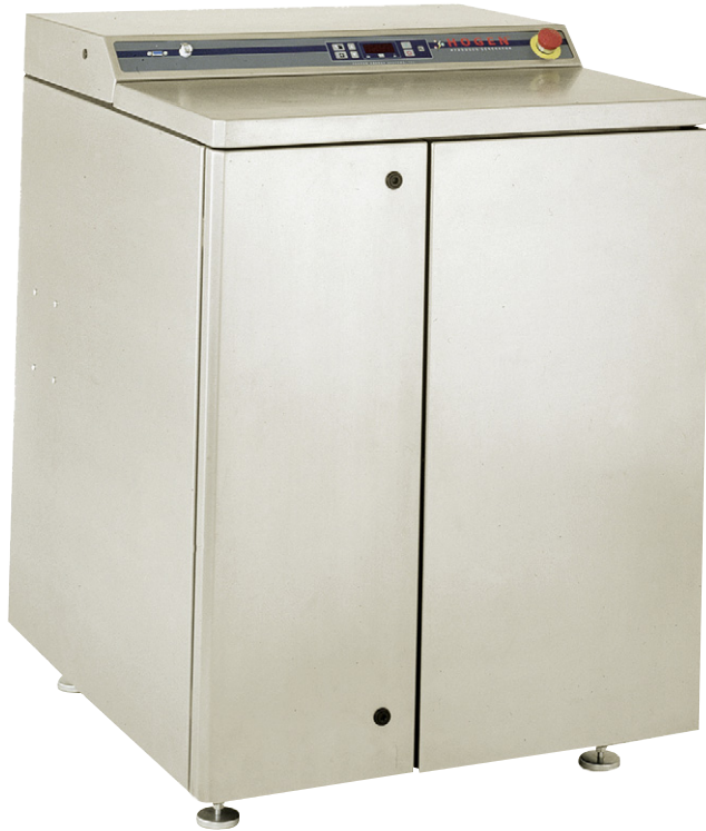
FIGURE 2.14 PEM electrolyzer HOGEN S Series by Proton OnSite. Productivity, 1\text{ m}^3\text{H}_2/\text{h} ; electric power consumption, 5.6\text{--}9.0\text{ kWh/m}^3 ; electrolysis voltage, 2.3\text{--}3.8\text{ V} ; output pressure, 1.4\text{ MPa} ; size, 97 \times 78 \times 10^6\text{ cm}^3 ; weight, 215\text{ kg} . (For color version of this figure, the reader is referred to the online version of this book.)
