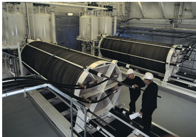
FIGURE 2.8 Alkaline water electrolysis modules developed by NEL Hydrogen. (For color version of this figure, the reader is referred to the online version of this book.)
