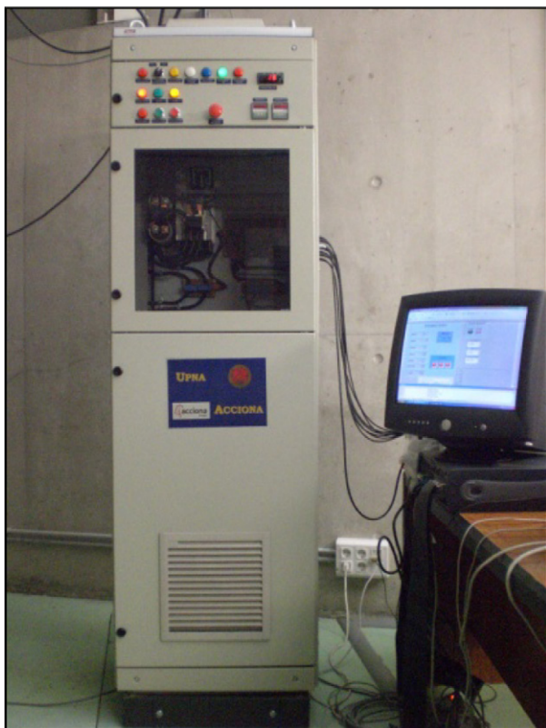
FIGURE 14.17 Electric power supply designed and developed by the authors for the study and analysis of electrolyzers. (For color version of this figure, the reader is referred to the online version of this book.)
